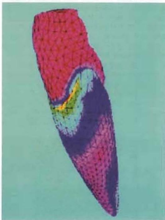
Figure 7 A computer model of stresses in a human tooth used for orthodontic research. (Photo, J. Middleton.)
